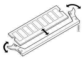
Figure 49 DIMM Socket with Single Release Lever
